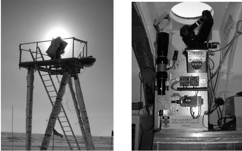
**Fig. 4.** Left picture: AFOS and ADIMM installed on the GMOUNT at the South Pole. Right picture: MASS and feed optics installed inside the AASTINO at Dome C.
