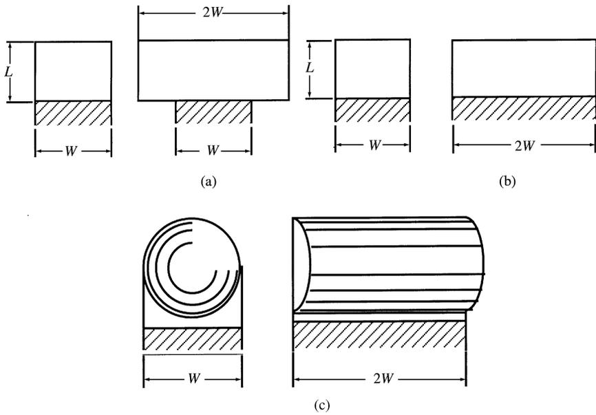
Figure 3. Plates of various sizes and shapes used to measure aerodynamic damping; (a) in stationary surrounding; (b) and (c) in the wind tunnel.
