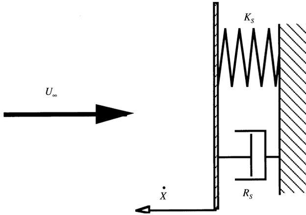
Figure 2. Schematic of the theoretical model of the plate oscillation in air flow.
