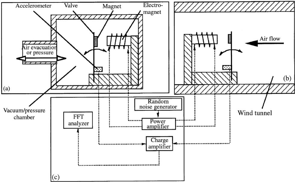
Figure 4. Schematic of the experimental set-up: (a) measurements in stationary air using vacuum/pressure chamber; (b) measurements in the wind tunnel; (c) instrumentation.
