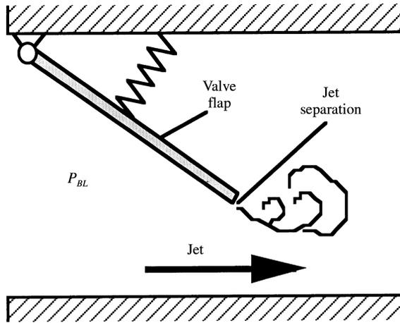
Figure 1. Schematic of blown-open pressure-controlled self-oscillating valves, where  $P_{BL}$  is the upstream blowing pressure.
