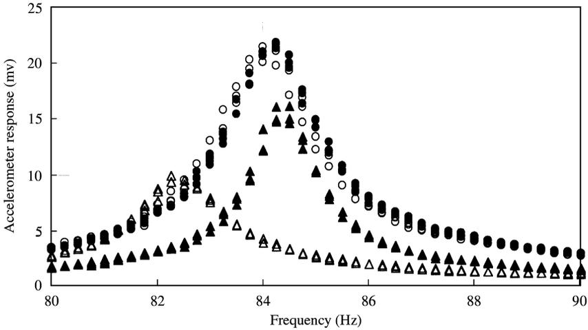
Figure 5. Experimental frequency response resonance curves of plates of various sizes oscillating in stationary air for various absolute pressure. ● Plate, 35 mm × 30 mm;  $P = 1$  kPa; ○ Plate, 35 mm × 30 mm;  $P = 800$  kPa; ▲ Plate, 70 mm × 30 mm;  $P = 1$  kPa; △ Plate, 70 mm × 30 mm;  $P = 800$  kPa.
