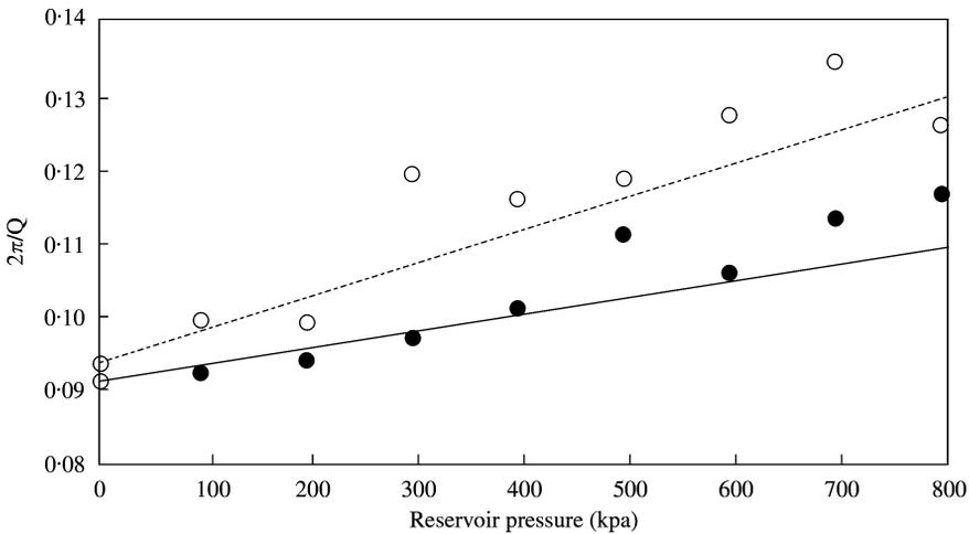
Figure 6. Variation of aerodynamic damping of oscillating plates in stationary air with absolute pressure. ●, experiments with plate 35 mm × 30 mm; ○, experiments with plate 70 mm × 30 mm; —, equation (11) (plate 35 mm × 30 mm); - - - - -, equation (11) (plate 70 mm × 30 mm).
