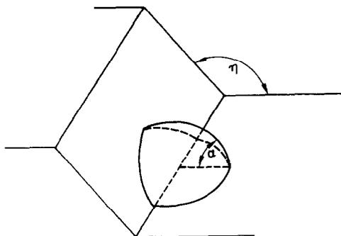
FIG. 1. Nucleus with contact angle  $\alpha$  on a step of angle  $\eta$ .
