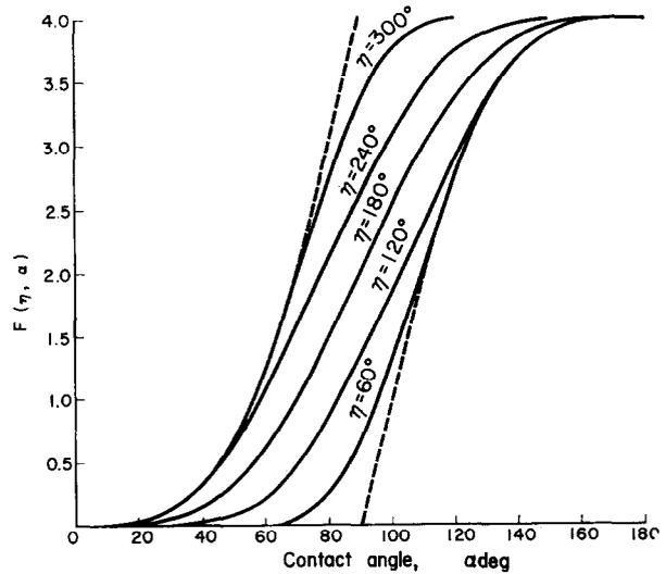
FIG. 4.  $F(\eta, \alpha)$  as a function of contact angle for representative values of step angle.
