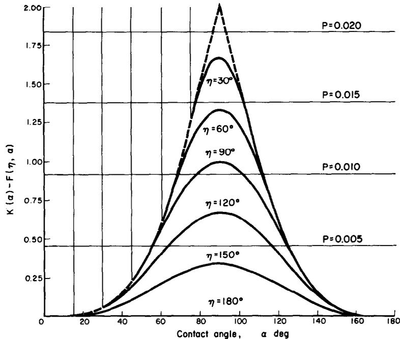
FIG. 5. Difference between the geometrical factor on a flat surface,  $K(\alpha)$ , and that on a step of angle  $\eta$ ,  $F(\eta, \alpha)$ , as a function of contact angle for representative values of step angle.
