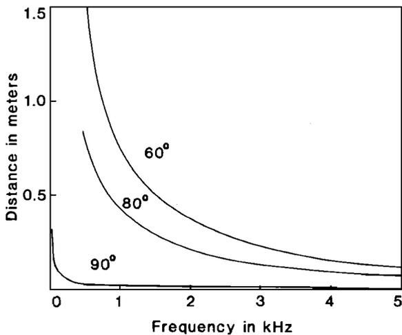
FIG. 4. Distance to the first zero of  $\xi(r)$  when  $\xi(0)$  is a maximum for cones of semiangle  $60^\circ$ ,  $80^\circ$ , and  $90^\circ$  (a flat plate).
