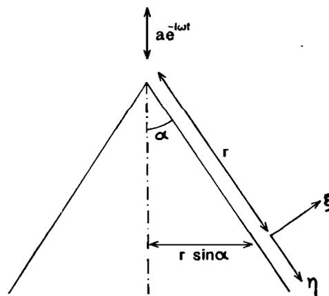
FIG. 1. Coordinate definitions for the conical shell.
