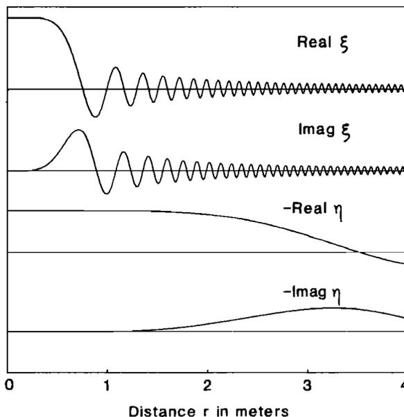
FIG. 3. Real and imaginary parts of the transverse and longitudinal wave displacements  $\xi$  and  $\eta$  on a conical shell of semiangle 60° at frequency 1000 Hz at the instant when displacement is a maximum at the apex  $r = 0$ . Both  $\xi$  and  $\eta$  are always real at the apex.
