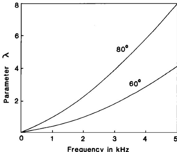
FIG. 2. Values of the parameter  $\lambda$  minimizing the mean-square solution error  $Z$  for brass conical shells of semiangle 60° and 80°, respectively.
