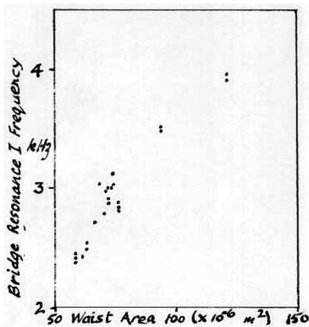
This figure shows the change in rocking frequency with change in the area of the waist region of the bridge. A narrow waist with reduced stiffness lowers the frequency; a wide waist raises the frequency. A resonance frequency of 3 kHz corresponds to a waist area of about  $70 \times 10^{-6} \text{ m}^2$ .
