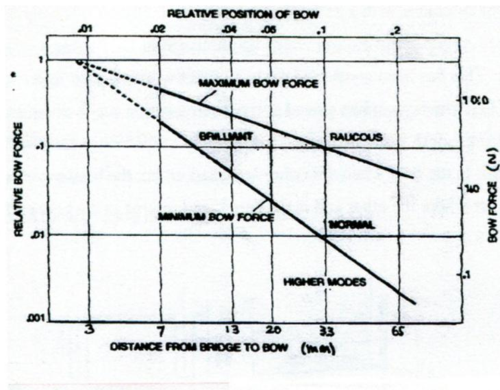
This figure shows the approximate bowing parameter limits for a violin. Brilliance is related to the increase in the number of harmonics in the sound. The latitude near the bridge is lower than near the fingerboard.
