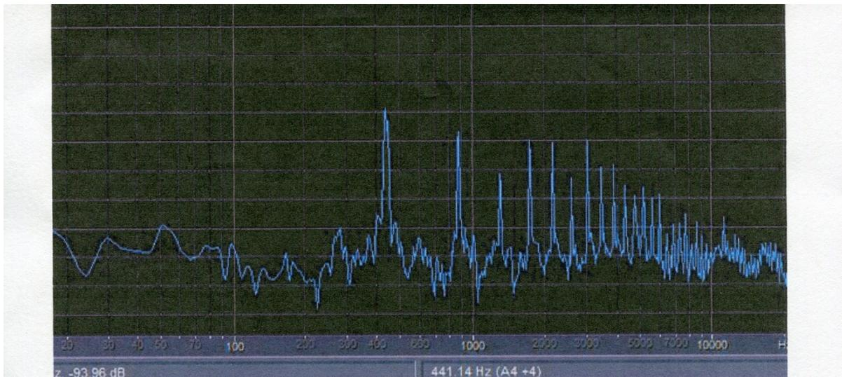
This figure shows the harmonic content of the open A string bowed 25 mm from the bridge with a force of 1.7 N. The height of the harmonics is influenced by the body response and will not show the progressive decrease in height mentioned above.
