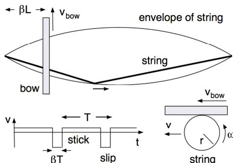
**Figure 1.** Helmholtz motion. The parabolic curves are the envelope traced by the Helmholtz corner (the kink in the string), which here travels anticlockwise. The graph shows the string speed  $v$  at the bowing point. The sketch at lower right shows a string with finite radius.
