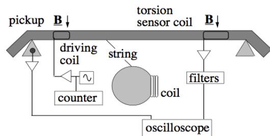
**Figure 3.** Two coils are glued to the side of the string, as shown in the inset. The magnetic field, provided in each case by permanent magnets, is perpendicular to the string and parallel to the plane of the coil. One coil (left) drives torsional waves and the other (right) detects them.
