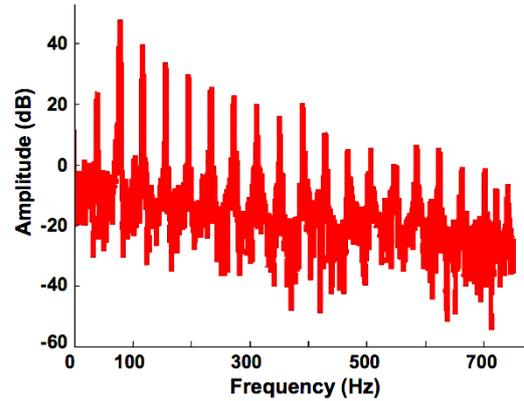
**Figure 9:** The spectrum of the steady-state bridge pick-up signal for the open string, bowed by the investigators in the lab.
