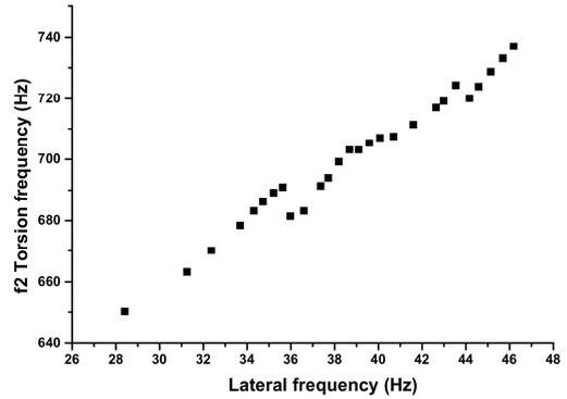
**Figure 6.** The frequencies of the first and second torsional resonances are plotted against that of the first translational resonance for a gut E1 string.
