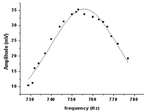
**Figure 7.** The amplitude of the first and second torsional modes of a wound steel E1 string (Flexocor) plotted against the frequency of the magnetic field producing the torsional motion (as shown in Figure 3). The continuous lines indicate the best fit to a Lorentzian.
