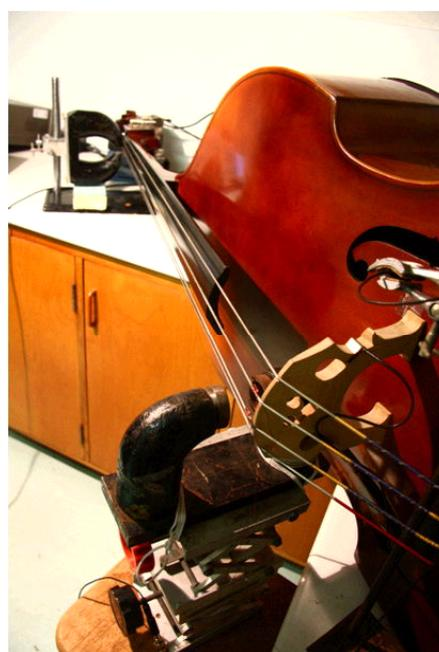
**Figure 4.** This photograph shows the apparatus for resonance measurements. Three different types of E1 string were studied: D’Addario Helicore orchestral medium H614, Pirastro Flexocor medium, both multi-core wound steel and an Efrano plain varnished gut E #450, a twisted, multistrand, gut string.
