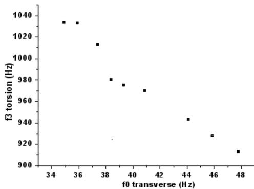
**Figure 5.** The frequencies of the first three torsional resonances are plotted against that of the first translational resonance for a wound steel E1 string (Flexocor) when the tension was varied.
