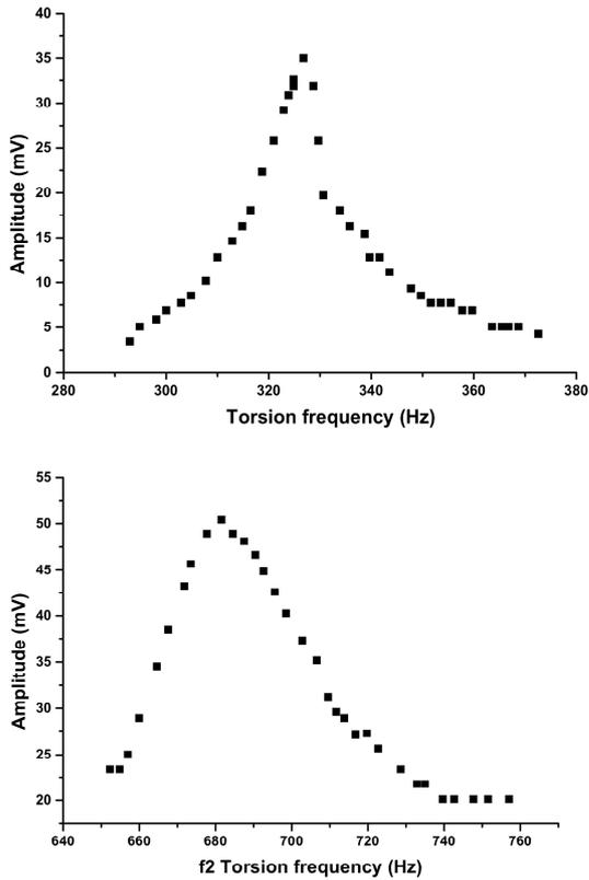
**Figure 8.** The amplitude of the first and second torsional modes of a gut E1 string as a function of frequency.
