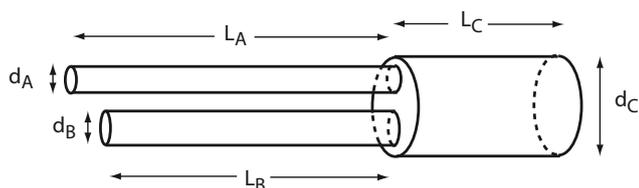
Figure 2. Schematic diagram used for the numerical model of the forked didjeridu measured in this study. Although the diameter  $d_C$  is greater than  $d_A + d_B$  in this sketch, this is not necessarily true in the model.
