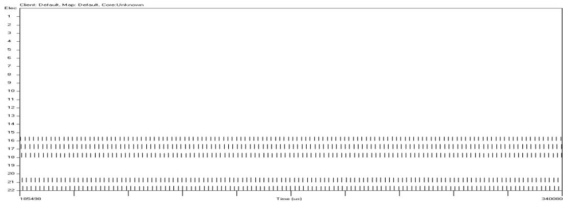
**Figure 9-1 Electrodegram of a constant rate strategy: Pitch is elicited by place information (Electrode) and temporal amplitude modulations below 187Hz (x tick is ~0.015s)**
