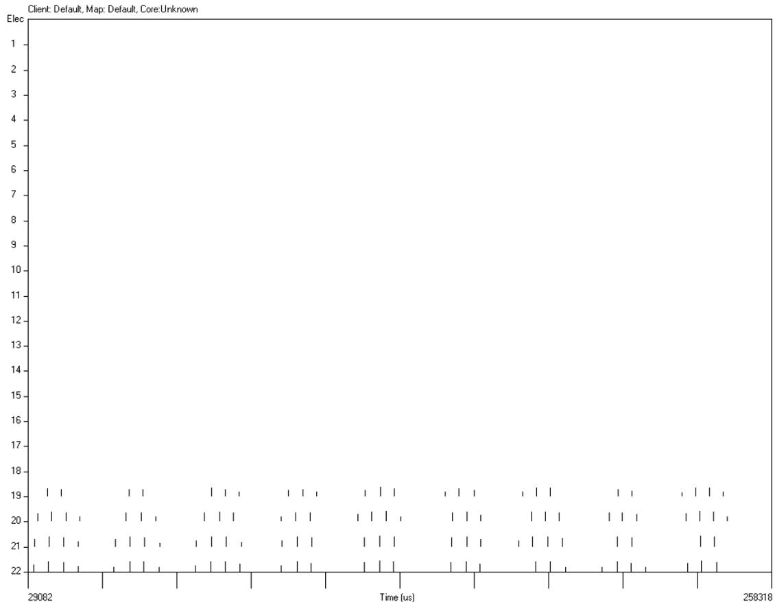
**Figure 9-15 2 Sine waves, close in frequency 200 Hz and 240 Hz. The stimulation rate is 200Hz and is amplitude modulated at the difference frequency of 40Hz (x tick is ~0.02s).**
