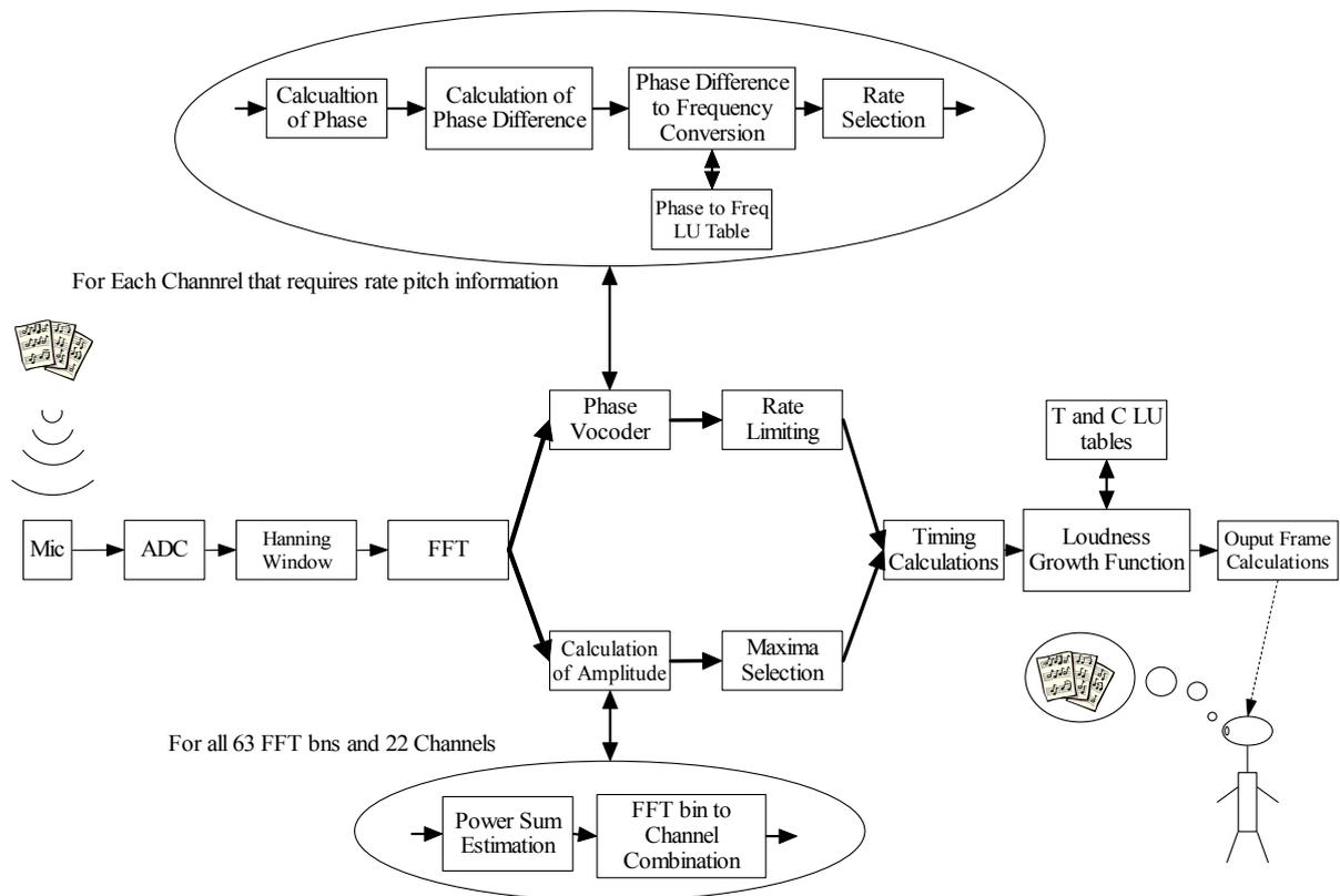
Figure 9-3 System diagram of Music-L signal processing scheme
