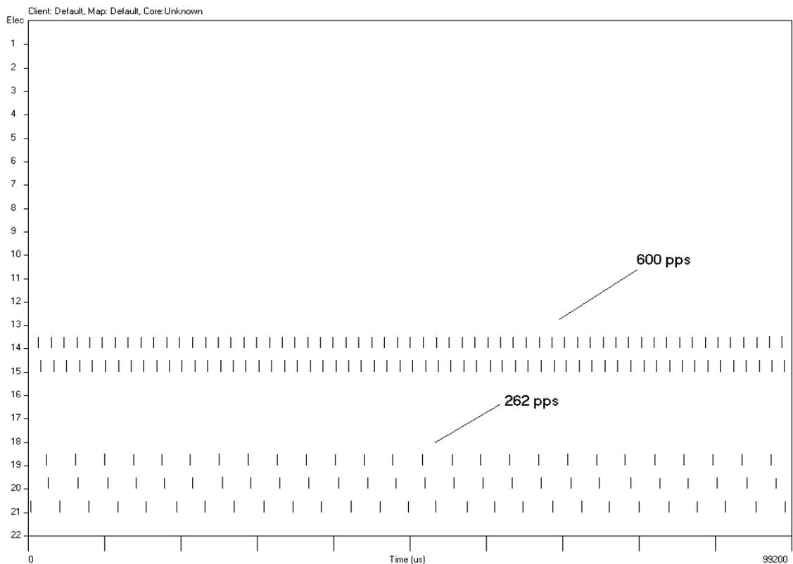
**Figure 9-12 Sine wave input of 262 Hz and 600Hz (x tick is ~0.01s).**
