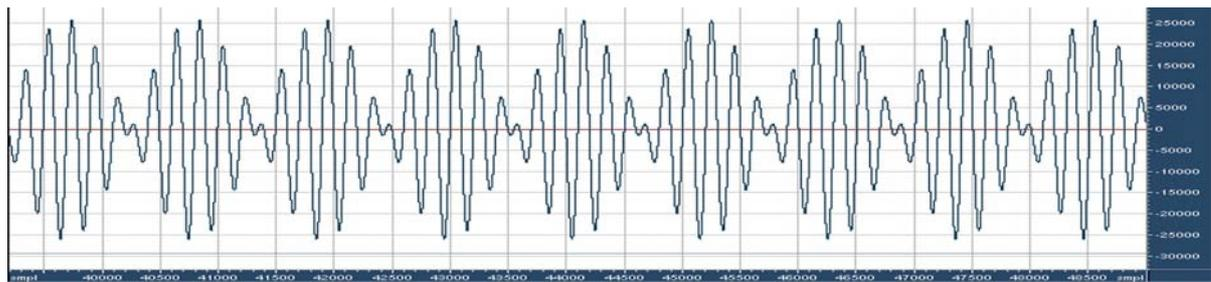
**Figure 9-14 Combined 200 and 240Hz sine waves.**
