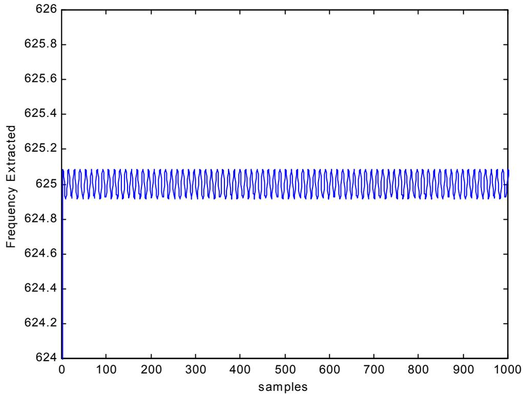
**Figure 9-8 Phase vocoder output in response to a 625Hz (center frequency of bin 6) sine wave. The maximum error is of the order of 0.1Hz.**
