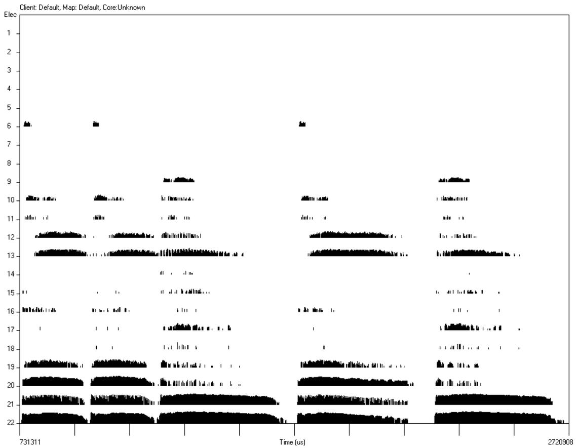
**Figure A-11-3** Electrodiagram of the phrase used in the Happy Birthday version of the test. This recording is with the last note that was selected by the CIR as the correct note (x tick is ~0.2s).
