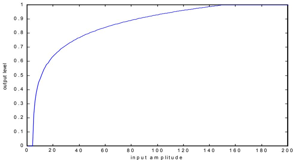
**Figure 9-11 Loudness growth curve mapping input amplitude to output current level**
