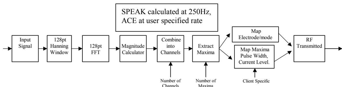
**Figure 2-1 Block diagram of ACE and SPEAK signal processing**
