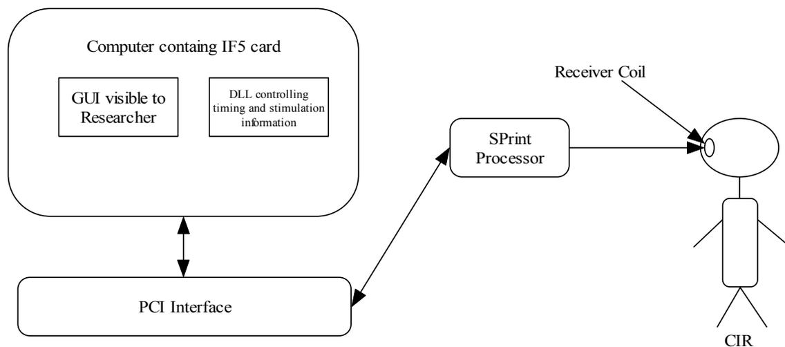
**Figure 3-2 Block diagram of system used for this experiment.**
