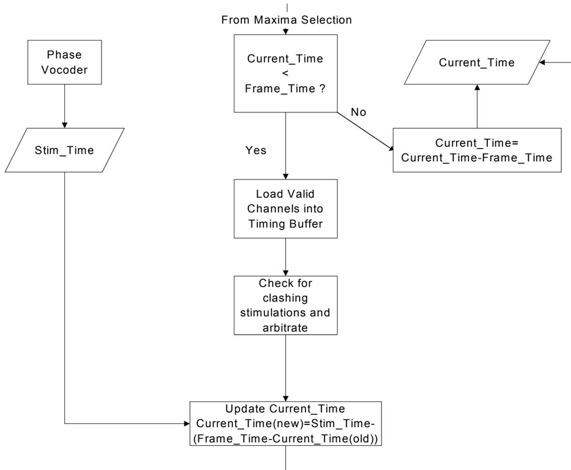
**Figure 9-10 Flow diagram of how timing is calculated**
