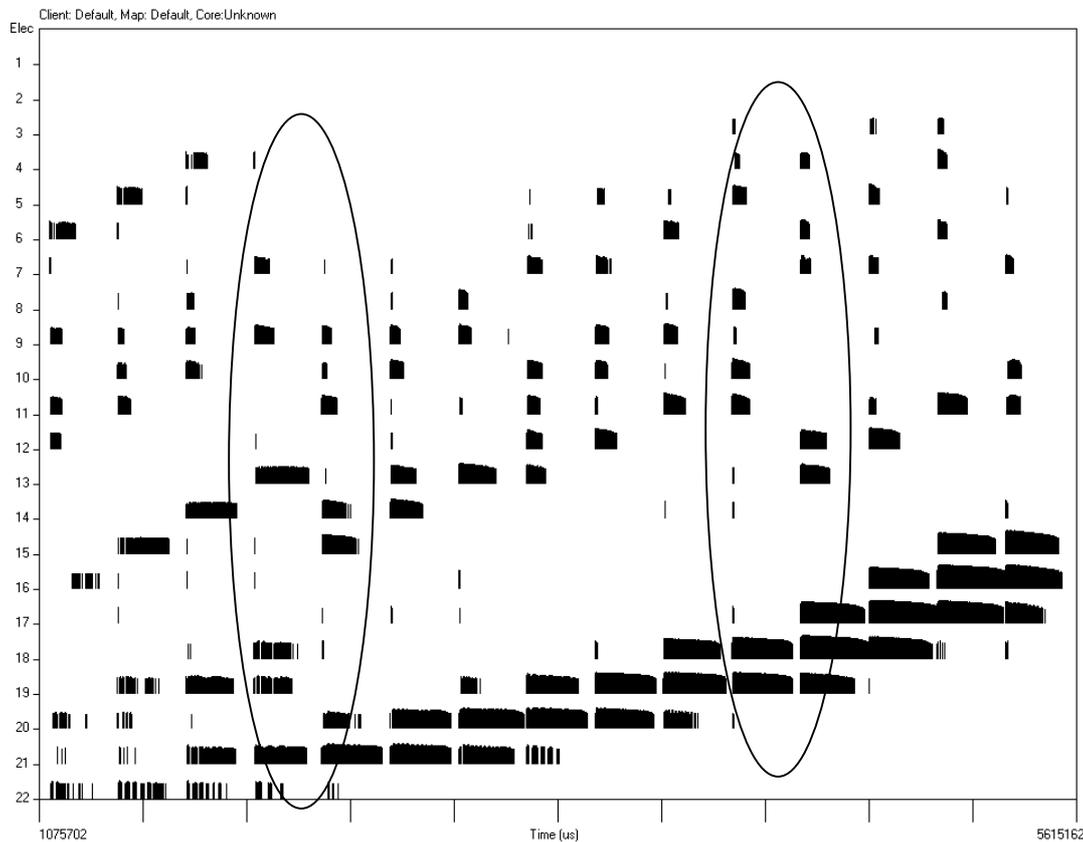
**Figure 8-6** Electrodegram showing how a peak picking algorithm can present ambiguous information about the pitch (x tick is  $\sim 0.45$ s).
