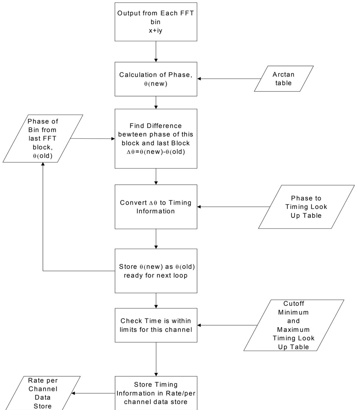
Figure 9-6 Block diagram of implementation phase vocoder
