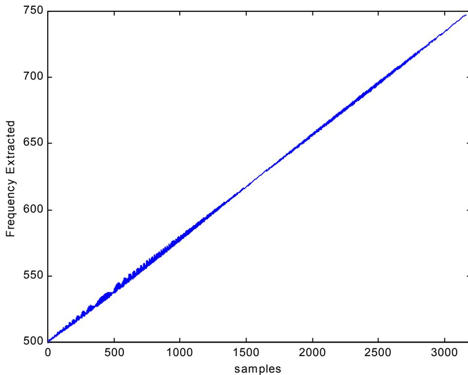
**Figure 9-9 Output of phase vocoder as frequency is swept between 500Hz and 750Hz**
