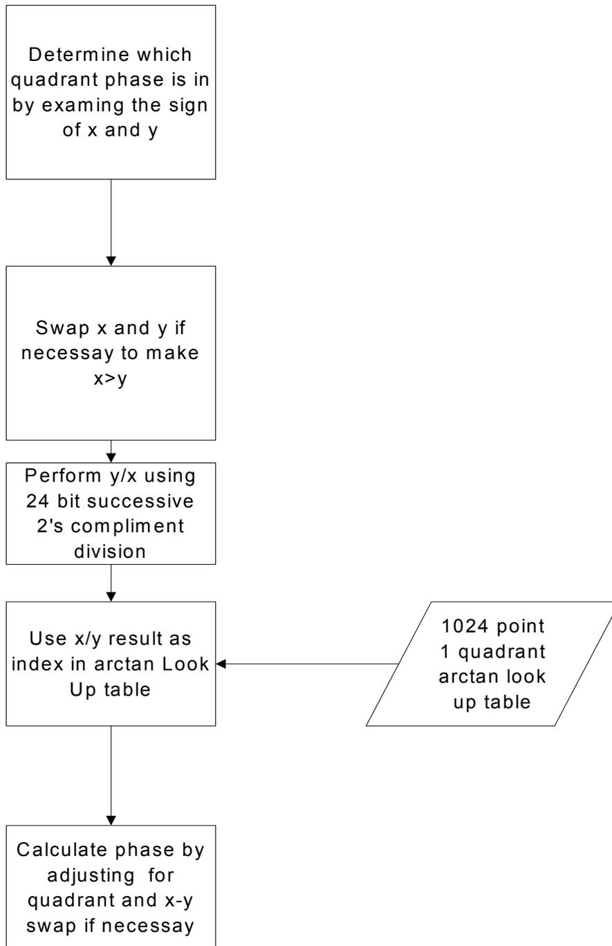
Figure 9-7 The 'Calculation of Phase' block from Figure 9-6 in detail
