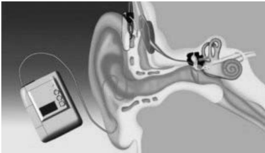
**Figure 1-6 Components of the cochlear implant system: The internal coil, integrated circuit and electrode and external microphone and body worn processor.**
