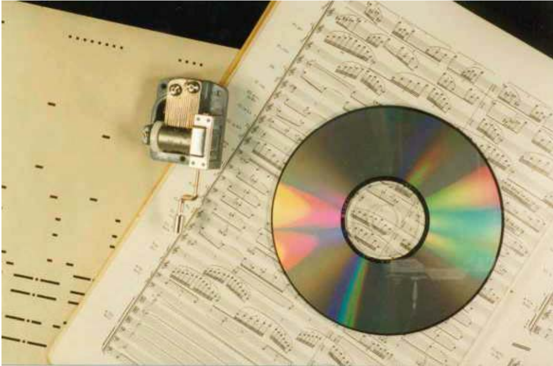
Fig. 1. Four digital storage media. (a) The cylinder and comb from a music box play 16 bars from Lara's Theme (M. Jarre). The 18 tines of the comb have different masses and thus play different notes when struck by spikes on the cylinder. It has 18 parallel channels—circles round the cylinder. The loudness is binary (spike or no spike, note or no note). The timing is in principle analog, but is here quantised in multiples of 1/12 of a bar. The uncompressed data content of this cylinder is therefore 18 \times 12 \times 16 = 3456 bits. (b) The pianola roll in the background also has parallel binary channels, but the length of the hole determines the time the strings sound before the damper is replaced. In that sense, both duration and timing could be analogue, but again they are quantised in this example. The uncompressed data content is 35,000 bits per metre. (c) Standard Western music notation is (largely) parallel binary digital coding: each line and space (parallel channels) represents a pitch, though that pitch can be varied by sharps and flats. The time coding is encoded digitally in symbols (see Fig 2). This example ( The Rite of Spring , I. Stravinsky) has about 30,000 bits on this page, which lasts a few seconds, using a coding somewhat like that in Fig 2c. (d) The CD also carries a binary digital signal (“pit” or “no-pit” in the track) but it is different in all other aspects. The signal is carried in serial rather than in parallel, and it encodes numbers that are proportional to the pressure of a sound wave. This CD records about 5 \times 10^9 bits, not counting error correction bits. The storage efficiencies are approximately: a) 5 \times 10^5 bit.kg -1 , b) 10^6 bit.kg -1 , c) 10^7 bit.kg -1 , d) 3 \times 10^{11} bit.kg -1 . The apparatus required for re-creation varies greatly in size: that for (a) is shown ( \sim 0.01 kg), that for (c) is \sim 10^4 kg, including the orchestra.
