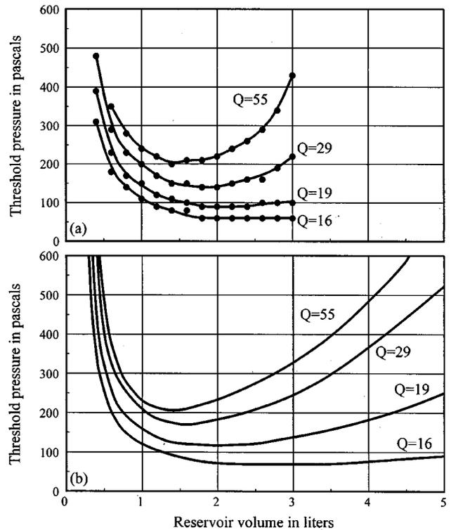
FIG. 2. (a) Measured threshold oscillation pressure of the experimental valve as a function of reservoir volume, with the  $Q$  value of the free valve flap as a parameter. For this valve the sheet thickness was 0.15 mm and the free resonance was 105 Hz. (b) Oscillation threshold as calculated from the theory.
