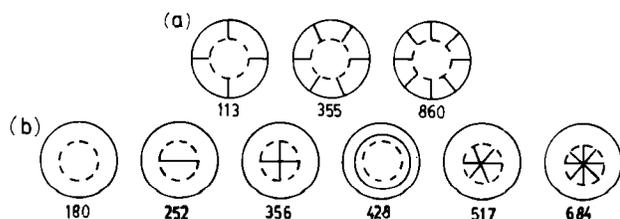
FIG. 8. Frequencies of five vibrational modes of a gold pan: (a) bell modes; (b) dish modes. The dashed circles outline the flat bottom.
