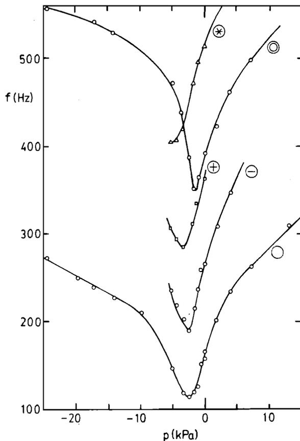
FIG. 9. Vibrational modes of a gold pan under static pressure.  $p$  is the air pressure inside the gold pan above and below atmospheric as in Figs. 5 and 6.
