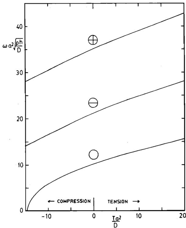
FIG. 1. Theoretical effect of radial tension and compression on the lowest vibrational frequencies of a flat circular plate (from data in Ref. 11).  $\omega$  is  $2\pi$  times frequency,  $a$  is the radius,  $\rho$  is density,  $h$  is thickness,  $D$  is stiffness, and  $T$  is tension.
