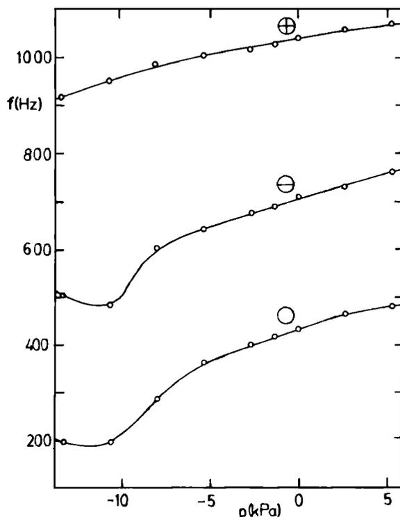
FIG. 6. Frequencies of three vibrational modes of a small Chinese opera gong under a static force.
