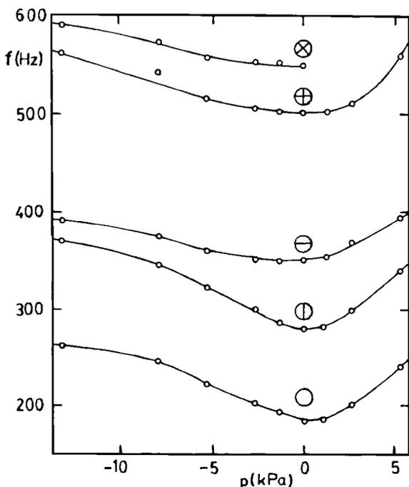
FIG. 5. Frequencies of five vibrational modes of a large Chinese opera gong under a static force.  $p$  is the air pressure inside the gong above and below atmospheric pressure.
