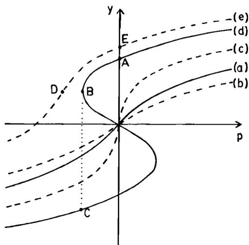
FIG. A1. Characteristic deformation curves under pressure  $p$  for a circular plate with fixed periphery: (a) unstressed; (b) with radial tension; (c) with radial compression; (d) with sufficient radial compression for dishing; (e) with inbuilt dishing stresses.
