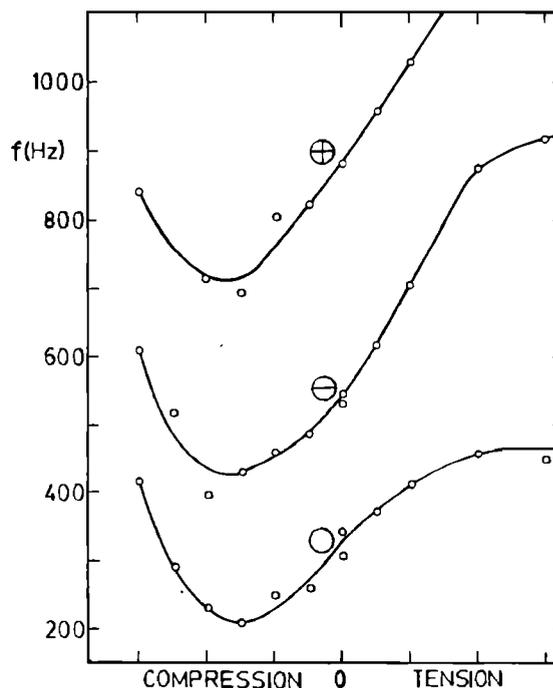
FIG. 7. Frequencies of three vibrational modes of a flat steel plate with radial compression or tension.
