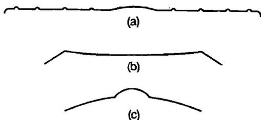
FIG. 2. Cross sections of (a) the Chinese tamtam, (b) the Turkish gong, and (c) the orchestral cymbal, referred to in this study. The diagrams are only approximately to scale.
