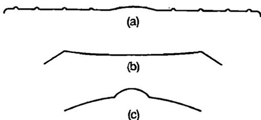
FIG. 2. Cross sections of (a) the Chinese tamtam, (b) the Turkish gong, and (c) the orchestral cymbal, referred to in this study. The diagrams are only approximately to scale.
