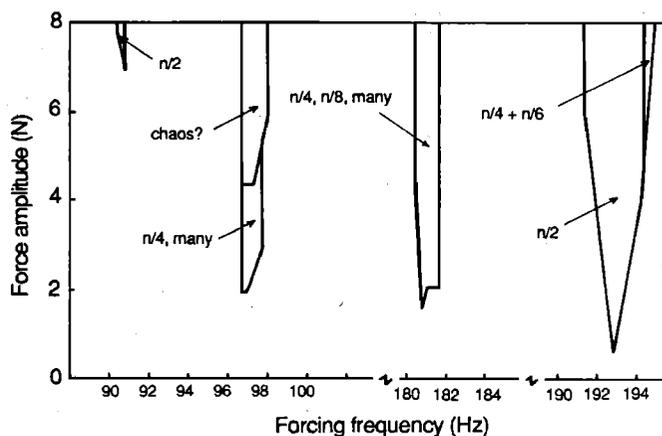
FIG. 4. Plot of the regions in (frequency, force) space for which complex behavior was found for the Turkish gong. The excitation frequency is, in each case, close to one of the major admittance maxima, near 96 and 200 Hz, respectively.
