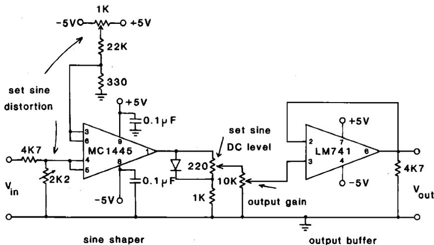
FIG. 8. Details of the shaping circuit used to convert triangular waves to sine waves in the system of Fig. 7. Adjustment of the signal level is critical to good operation. (Original source of circuit is not known.)
