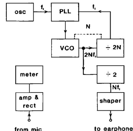
FIG. 7. Schematic circuit for a simple harmonic generator and measurement system. The principle of operation is described in the text.
