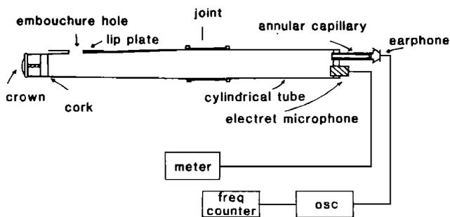
FIG. 1. Schematic section of a typical flute head joint with the impedance head and measuring equipment in place. An alternative simplified electronic system is shown in Fig. 7.
