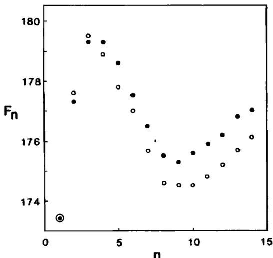
FIG. 4. Measured resonance signatures  $F_n$  of a student flute head joint (filled circles) and of a simple conical head joint (open circles). Each was fitted to a cylindrical tube to give a fundamental resonance near 170 Hz and the curves have then been displaced vertically to coincide at that point ( $n = 1$ ).
