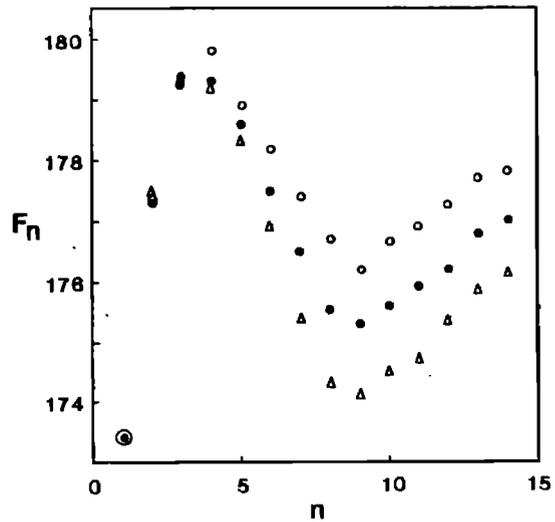
FIG. 5. Signature curves  $F_n$  for a typical student flute head joint with cork position set at 15 mm $\circ$ , 17 mm $\bullet$ , and 19 mm $\Delta$  from the center of the embouchure hole.
