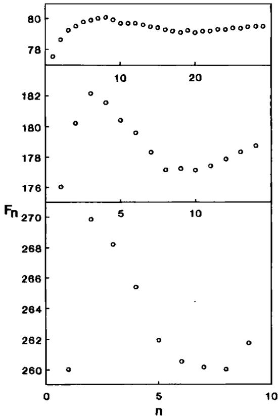
FIG. 3. Measured resonance signatures  $F_n$  for a conically tapered head joint attached to a length of cylindrical tube so as to give a fundamental frequency of about (a) 80, (b) 176, and (c) 260 Hz.
