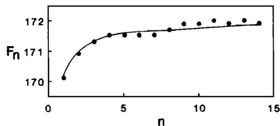
FIG. 2. Measured resonance signature  $F_n$  for a simple cylindrical tube 19 mm in diameter and about 50 cm long. The curve is calculated from theory for a smooth tube.
