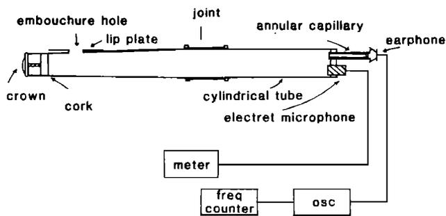
FIG. 1. Schematic section of a typical flute head joint with the impedance head and measuring equipment in place. An alternative simplified electronic system is shown in Fig. 7.
