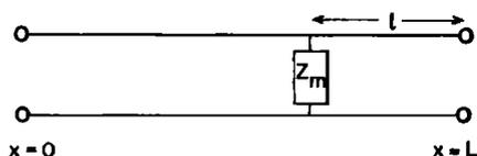
FIG. 6. Electric transmission line analog for a flute head joint. The impedance is measured at  $x=0$ , the head is closed by a rigid stopper at  $x=L$ , and the embouchure hole appears as a shunt of impedance  $Z_m$  at a distance  $l$  from the stopper.
