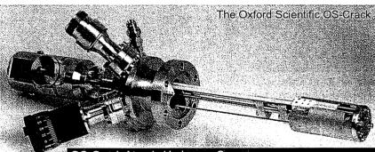
OS-Crack Atomic Hydrogen Source The Oxford Scientific OS-Crack uses e-beam heating of a tungsten capillary to thermally dissociate the gas passing through it, producing atomic hydrogen at >95% efficiency.
