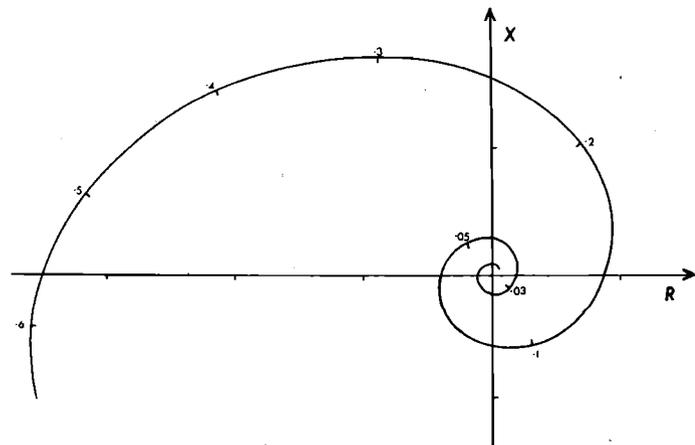
FIG. 2. Acoustic impedance  $Z=R+iX$  of the blowing jet of an organ pipe as described by Eq. 2. As discussed in the text, the impedance units are undetermined but the figure has been drawn the same size as Fig. 1 for qualitative comparison. The parameter on the curve is the blowing pressure in inches of water assuming a jet length of 7 mm, a sounding frequency of 440 Hz, and a wave-propagation velocity along the jet of 0.4 times the jet air velocity, again for comparison with Fig. 1.
