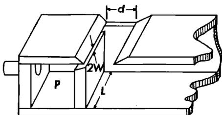
FIG. 4. Schematic diagram of the mouth of an organ flue pipe showing the jet thickness  $2W$ , jet width  $L$ , and lip cut-up  $d$ .
