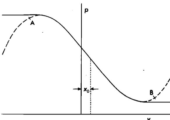
FIG. 3. Static interaction curve for a jet exciting an organ pipe. An acoustic particle velocity  $v$  out of the pipe mouth causes a pressure  $p$  due to interaction of the jet with the pipe lip.  $x_0$  is the static offset in the position of the jet relative to the lip, as defined in Sec. 6. The broken curve is a cubic approximation to the interaction curve, valid within the range A to B.
