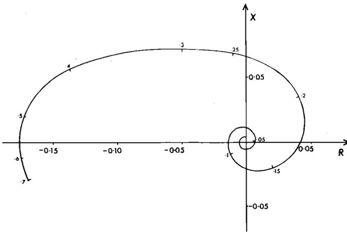
FIG. 1. Acoustic impedance  $Z=R+iX$  of the blowing jet of a flute as measured by Coltman<sup>3</sup> for a particular jet configuration. The impedance is given in units of the characteristic impedance of the tube, the parameter on the curve is the blowing pressure in inches of water, and the sounding frequency is 440 Hz.
