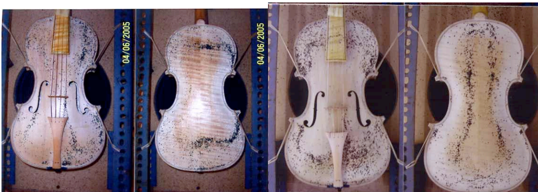
Figure 8.9 Baroque violin bridge and soundpost (4.3 @ 5/15) at f-holes. Left: B1-471 Hz. Right: B1+585 Hz.
