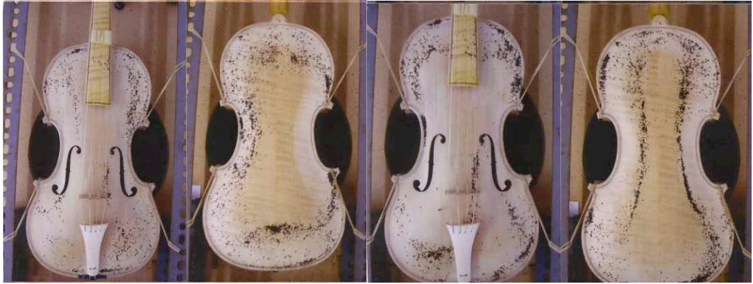
Figure 8.10 Baroque violin bridge below f-holes, soundpost at notches. Left: B1-478 Hz. Right: B1+610 Hz.
