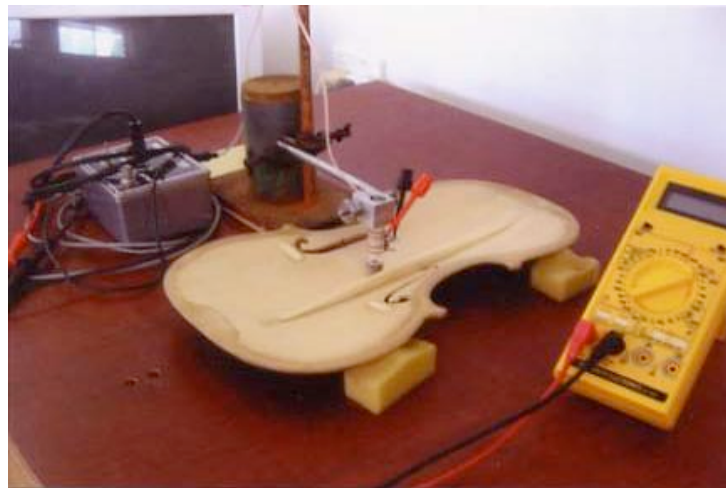
Figure 4.4 Setup for determining plate Chladni patterns and mode frequencies The magnet was placed in an anti-nodal position for each mode.
