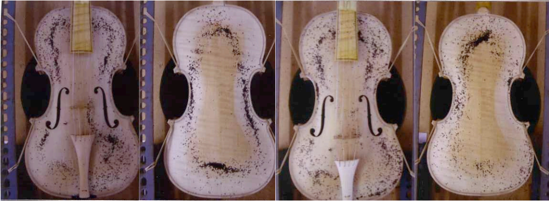
Figure 8.8 Baroque violin A0 280 Hz. Soundpost (4.3 at 7/15) at f-holes. Left: bridge at f-holes. Right: bridge below f-holes
