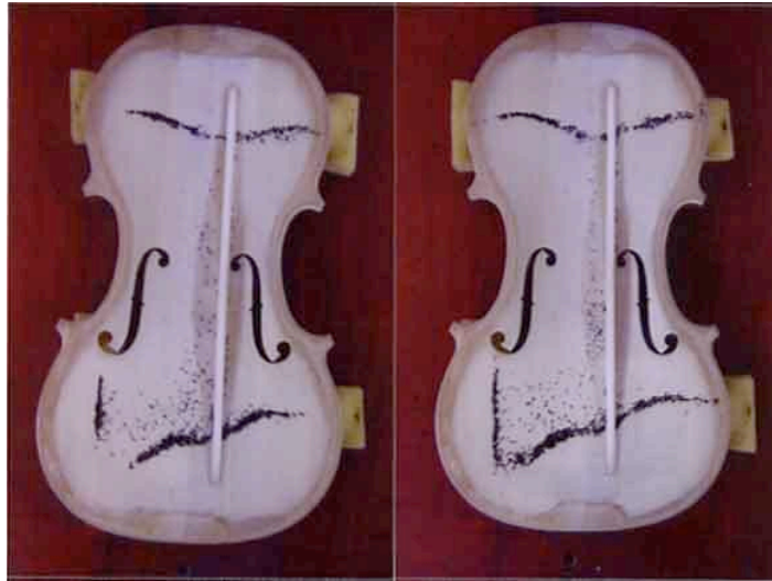
Figure 10.4 The top plate with new bassbar fitted #5 showing nodal line runout (left) and after retuning (right) with the result in Table 10.5
