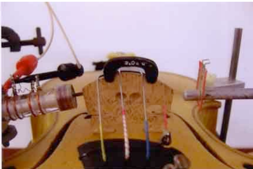
Figure 11.7 Violin setup for bridge rocking mode determination.
