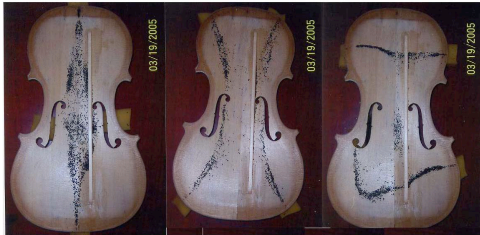
Figure 4.8 Top plate Chladni patterns on modes #1, #2 and #5 as finally fitted with bassbar tuned as shown in Tables 4.7 and 4.8
