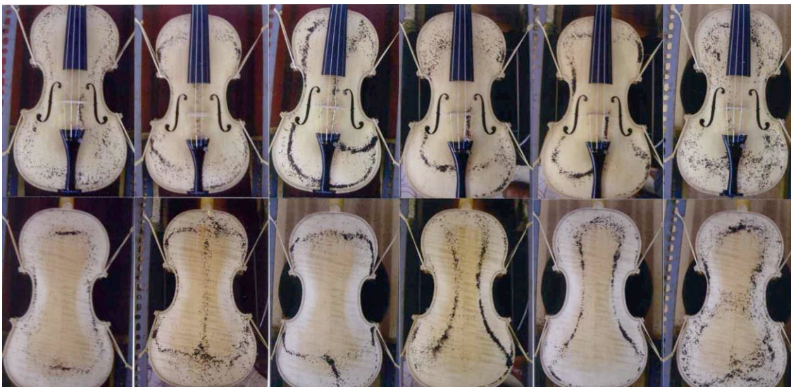
Figure 4.14 Idealised Chladni patterns (top) and photographs (below) for the vibration modes in the Romantic violin
