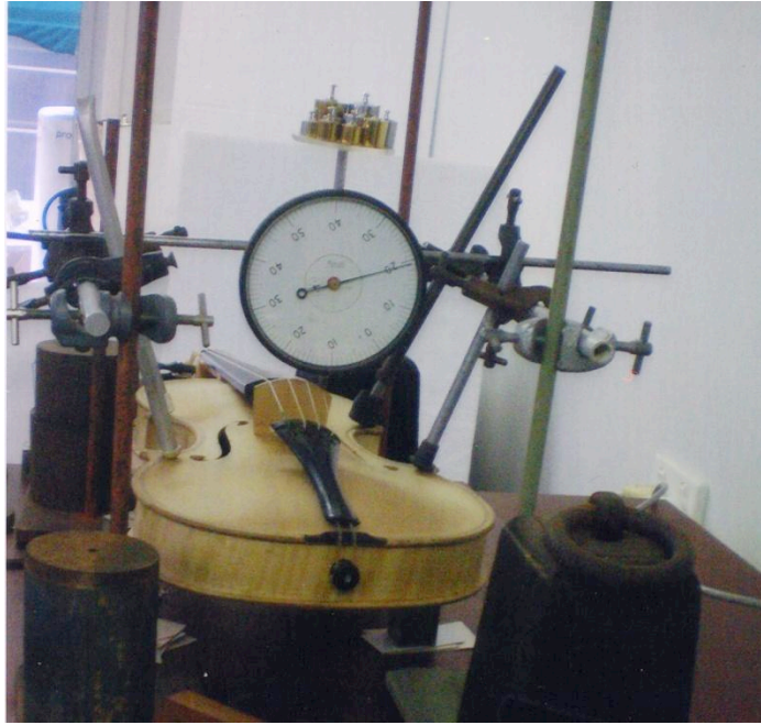
Figure 5.10 Setup for measuring the static stiffness as seen by the two feet of the bridge as shown in Table 4 (violin No 2)
