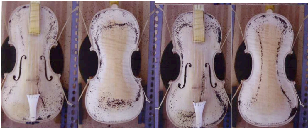
Figure 8.11 Baroque violin bridge and soundpost below f-holes. Left: B1-471 Hz. Right: B1+604 Hz.
