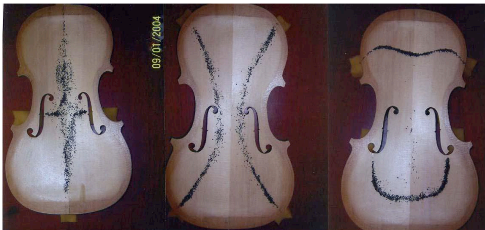
Figure 4.5 Top plate Chladni patterns of modes #1, #2 and #5 without a bassbar as described in Table 4.2
