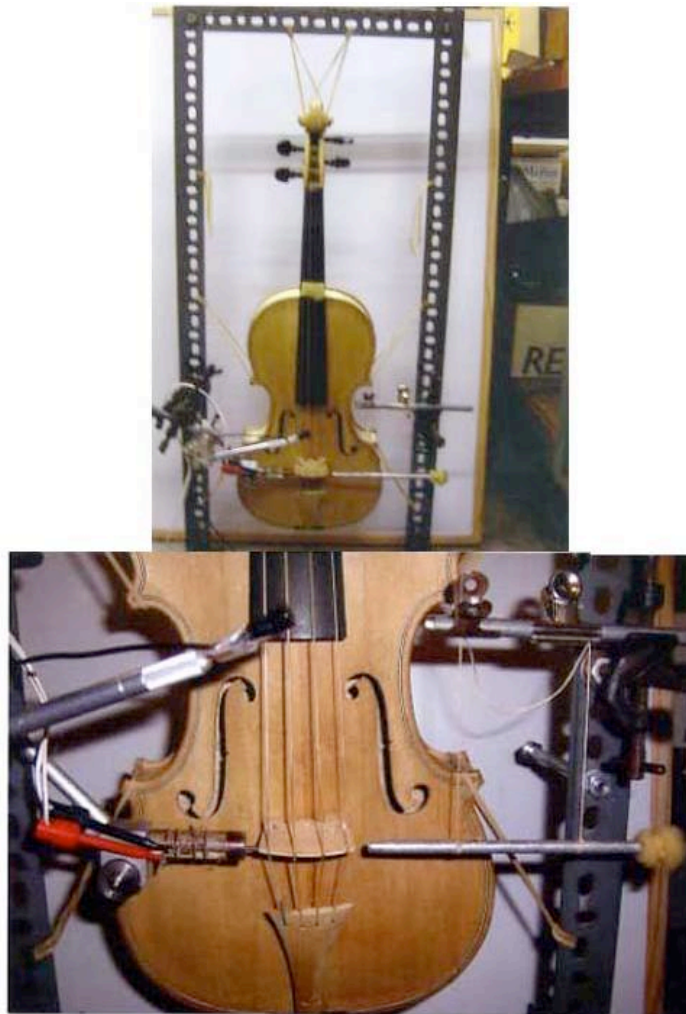
Figure 5.1 frame and rubber band suspension used for determining the tap response, showing pendulum bar, the microphone and the magnet/coil.
