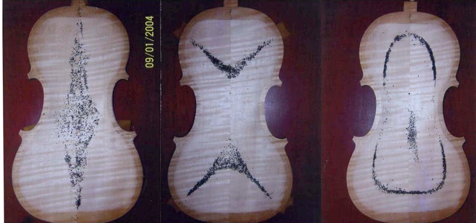
Figure 4.6 Back plate Chladni patterns of modes #1 #2 and #5 as shown in Table 4.2
