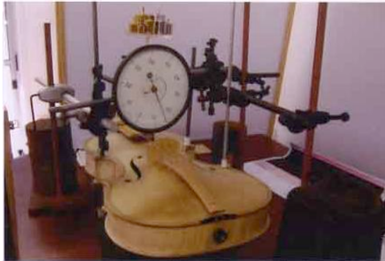
Figure 8.13 Measure of static stiffness of the baroque violin
