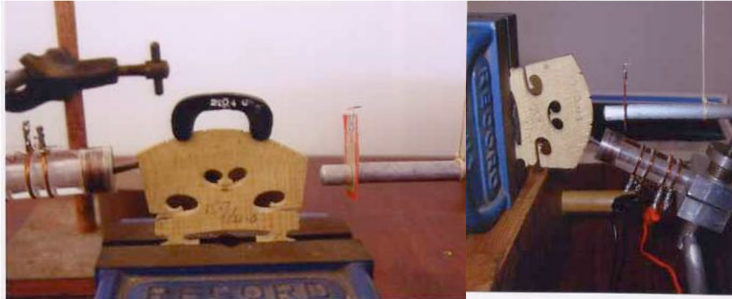
Figure 11.6 experimental setup to determine bridge resonances on a rigid base
