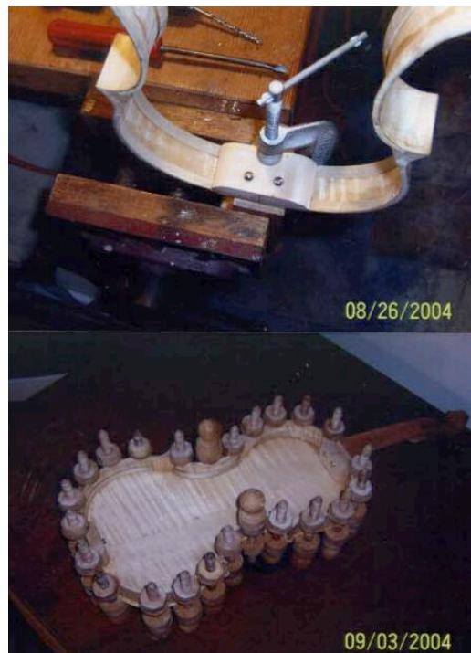
Figure 4.1 The method of attaching the neck to the sides and gluing on the back. The top and back were cut on the quarter and glued down the centre to make a “book joint” and give billets from which were carved the designed arching and thickness required for these parts.
