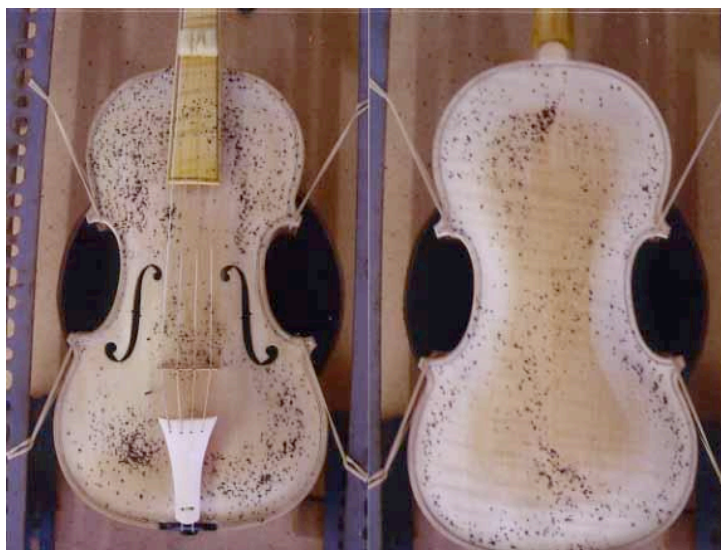
Figure 8.12 Baroque violin bridge below f-holes, soundpost at f-holes. Body mode at 875 Hz.
