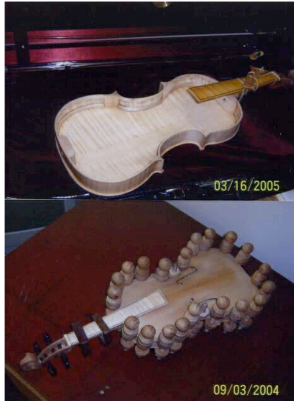
Figure 4.2 Attaching the Baroque fingerboard and gluing on the top
