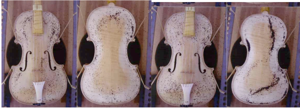
Figure 8.8a The Baroque violin with the bridge and soundpost below the f-holes. Left: A0 285 Hz. Right: 690 Hz.
