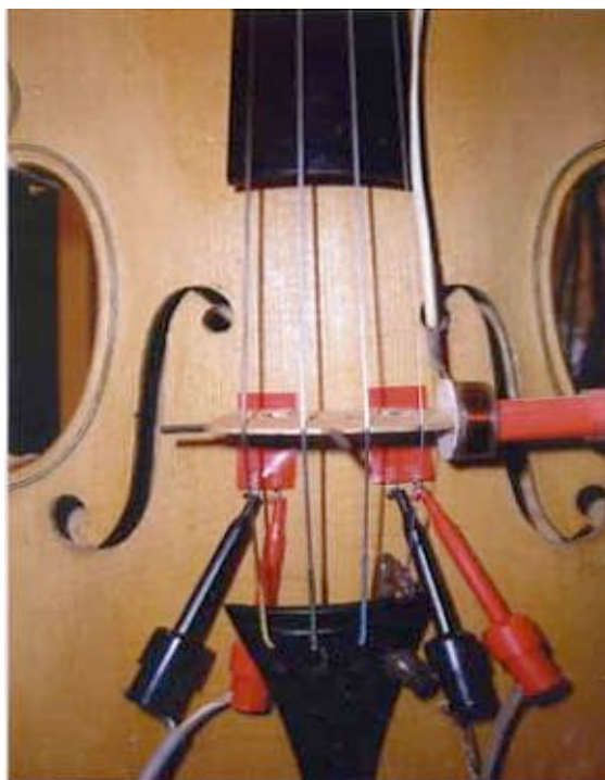
Figure 11.8 Setup with force transducers under the bridge feet. The bridge was driven by a coil attached to the treble edge.
