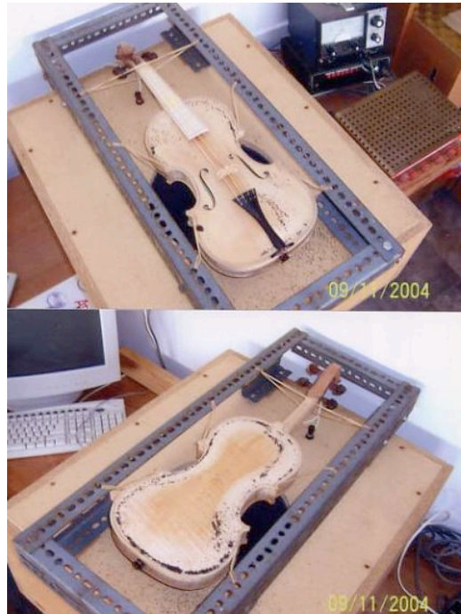
Figure 5.6 frame and rubber band suspension for determining Chladni patterns and resonance characteristic parameters
