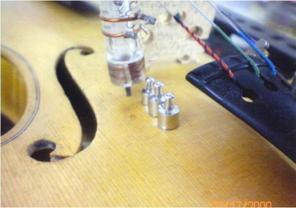
Figure 5.7 Arrangement of magnet/coil near the bass foot of the bridge and the placement of the added masses for determining df/dm .
