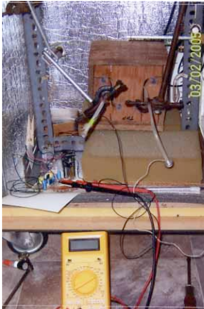
Figure 9.1 Two litre box with f-holes cut into a 3.5 mm insert for determining the Helmholtz resonance showing microphone (left) connected to a DVM via an amplifier and an exciter (right) connected to a signal generator/amplifier.
