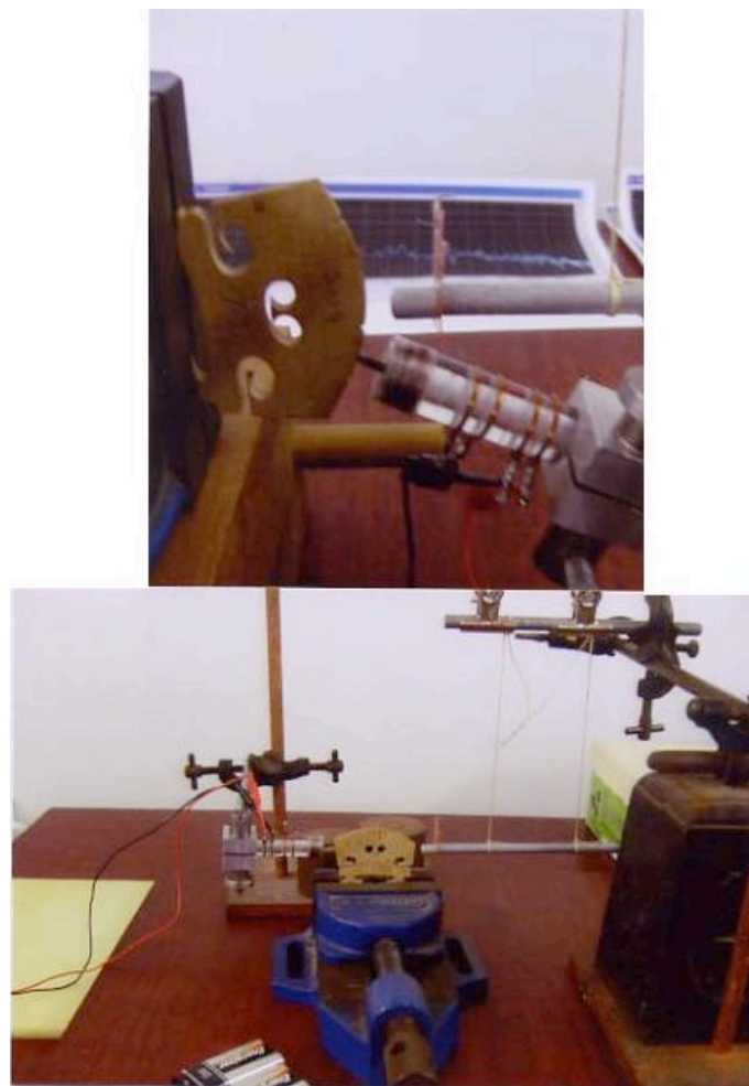
Figure 5.11 Setup for measuring the rocking resonance at about 3 kHz for a modern bridge mounted on a firm base
