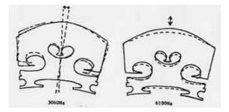
This figure illustrates the in-plane motion of two resonances of the violin bridge. On the left, the rocking motion of the upper part above the waist at 3 kHz, on the right, a vertical motion at 6 kHz.
