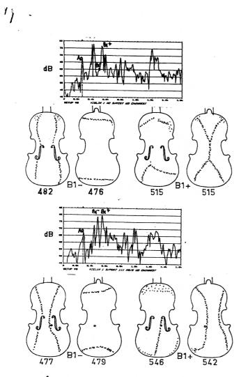
This figure shows an example of the effect on the mode shape with and without the soundpost for the two body resonances near 500 Hz. The tap response with no soundpost shows a small peak for B1- which may be in error. The repositioning of nodal lines is quite evident. It is interesting that from the tables above, the radiation for B1- (15 kg/s) is greater than that for B1+ (5 kg/s) which makes the latter a better radiator.
