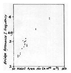
This figure shows the change in rocking frequency with change in the area of the waist region of the bridge. A narrow waist with reduced stiffness lowers the frequency; a wide waist raises the frequency. A resonance frequency of 3 kHz corresponds to a waist area of about 70 x  $10^{-6}$  m<sup>2</sup>.
