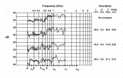
*Figure 1.* Saunders Loudness Curves for violin No 1 with soundposts located in the positions shown.
