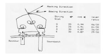
This figure shows the geometry of rocking about the treble foot for bowing on the D string.
