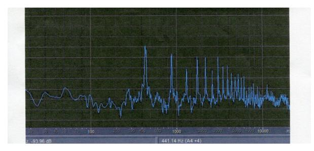
This figure shows the harmonic content of the open A string bowed 25 mm from the bridge with a force of 1.7 N. The height of the harmonics is influenced by the body response and will not show the progressive decrease in height mentioned above.
