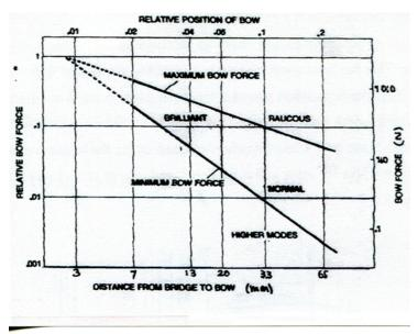
This figure shows the approximate bowing parameter limits for a violin. Brilliance is related to the increase in the number of harmonics in the sound. The latitude near the bridge is lower than near the fingerboard.
