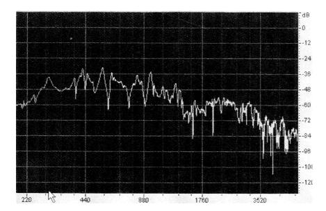
This figure illustrates the tap response of a modern violin showing the resonance peaks with the lowest peak being the main air resonance. The other peaks are body resonances. Between resonances of the same polarity there is a sharp trough. Resonances that have opposite polarity have a shallow trough e.g. the main air resonance and the next higher resonance.
