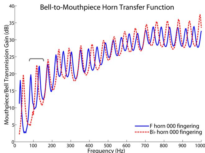
FIG. 2. (Color online) Bell-to-mouthpiece horn transfer function measured for the 000 fingering on the F and B $\flat$  horn (solid and dashed lines, respectively). The pale horizontal bracket indicates the nominal sounding range (F2-E3) of the 26 in. timpani used. Experimental configuration as shown in Fig. 1(A).
