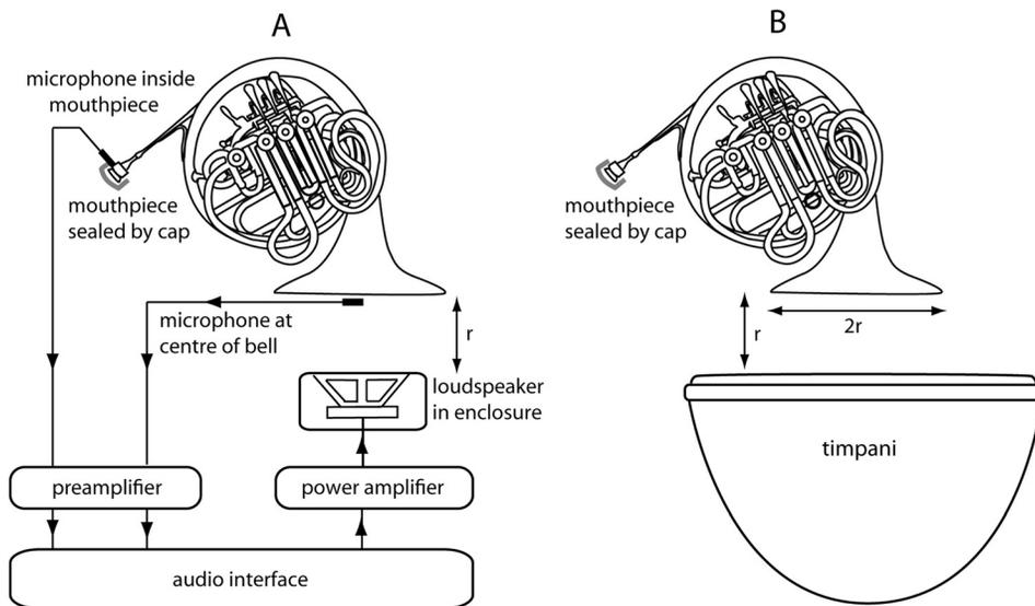
FIG. 1. Schematic diagram (not to scale) showing the experimental apparatus. (A) shows the configuration used for measuring the bell to mouthpiece transfer function. (B) shows the configuration used to measure the effect of timpani strokes on the pressure in the mouthpiece. For clarity the microphones in the mouthpiece and bell have not been shown in (B).
