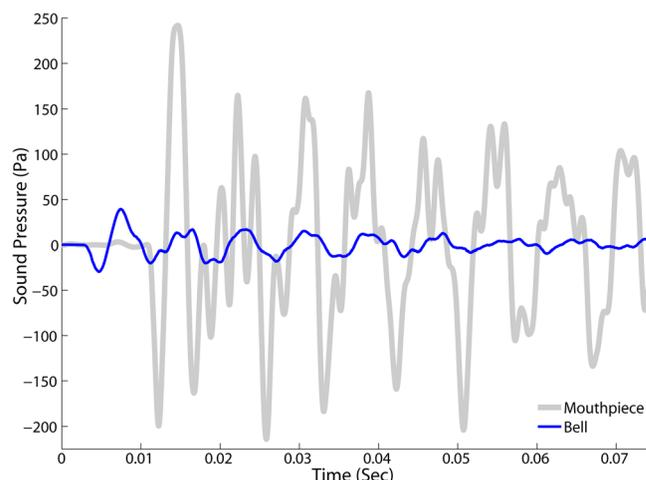
FIG. 3. (Color online) A typical waveform of the initial pressure pulse of a timpani stroke, nominally tuned A2 + 25 cents, measured in the bell (dark line) and in the mouthpiece (pale line) for the B $\flat$  horn 000 fingering. Experimental configuration as shown in Fig. 1(B).
