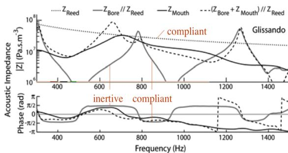
**Figure 17.** Measurements of the magnitude and phase of  $(Z_{\text{mouth}} + Z_{\text{bore}}) \parallel Z_{\text{reed}}$  and its components. A clarinetist was pitch bending on the clarinet (Chen *et al.*, 2009).
