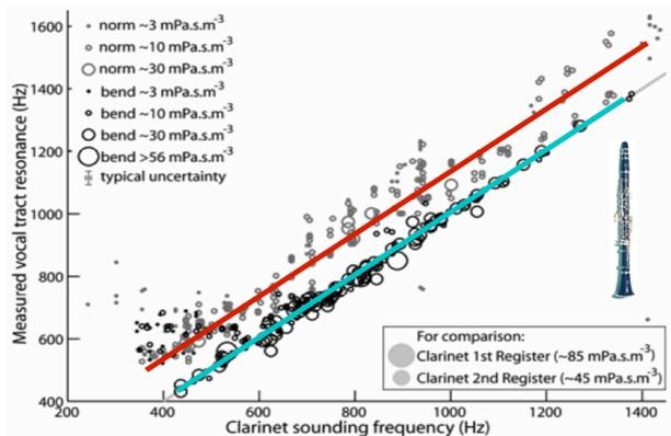
**Figure 16.** Frequency and magnitude of peaks in the vocal tract impedance, measured during playing the clarinet. The red line summarises typical playing in the clarino register while the green line summarises pitch bending in the same range.
