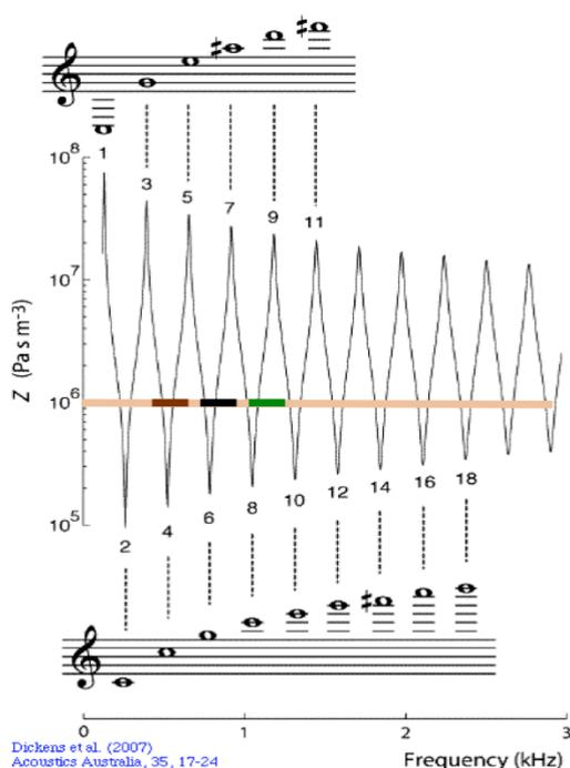
**Figure 4.** The measured impedance of a cylindrical pipe, 600 mm long and 15 mm in diameter, and open at the far end, the frequencies of maxima and minima are indicated as pitches (Dickens *et al.*, 2007a). A  $1 \text{ M}\Omega$  line is drawn on this and subsequent curves for reference.
