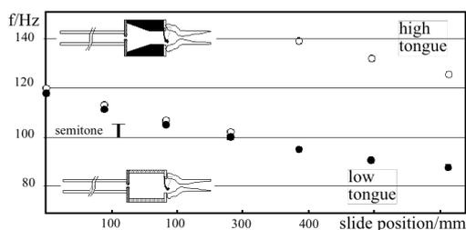
**Figure 12.** The playing frequency of an artificial trombone playing system as the slide is extended from the closed position (0 mm). The open filled circles refer to geometrically simplified ‘vocal tracts’ represented by the sketches for ‘high tongue’ (top) and ‘low tongue’ (bottom). From (Wolfe *et al.*, 2003).
