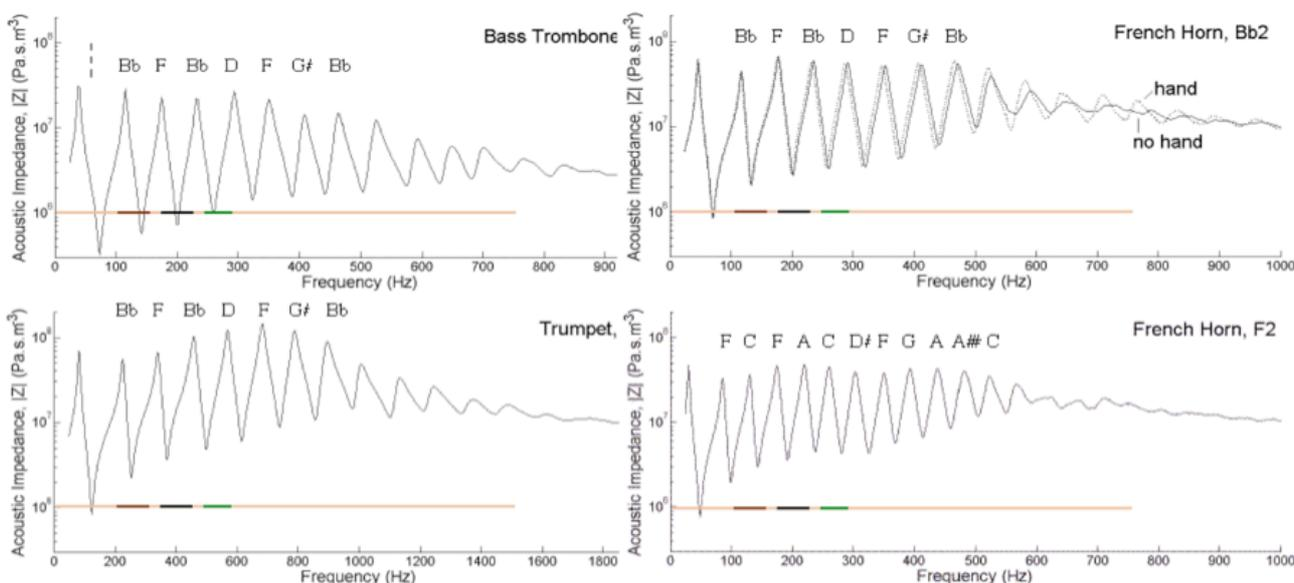
**Figure 7.** Measured acoustical impedances for brass instruments: a Bb bass trombone (first position, valve not depressed), a Bb trumpet (no valves depressed) and a horn in the open Bb and F configurations (no finger valves depressed) (Chen, 2009; Wolfe, 2005). The frequency scale for the trumpet is twice that of all the others, which shows that the trumpet is rather like a one-half scale model of the trombone: in Italian, *tromba* means trumpet and *trombone* means big trumpet.
