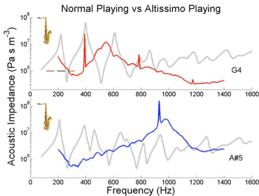
**Figure 14.** The broad, pale grey line shows the impedance of the bore for the fingerings that play G4 in the standard range of the tenor saxophone and A#5 in the altissimo range. (On this transposing instrument these notes are written A5 and C7.) The vocal tract impedance, measured while playing these notes is shown in red and blue respectively. The sharp peaks are harmonics of the note played; the broad peaks are resonances in the tract (Chen *et al.*, 2007).
