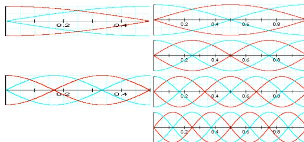
**Figure 5.** Standing waves in a cylinder. For the open-closed pipe (left) the pressure (red) has an antinode at the closed end (left) and a node at the open end. The open-open pipe has pressure nodes at both ends. These waves correspond (left) to the first two maxima in Figure 4, and (right) to the first four minima.
