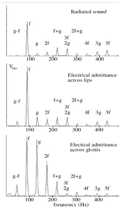
**Figure 11.** The spectrum of the radiated sound of a didjeridu vocalisation. The middle trace shows the MHz electrical admittance across the player’s lips, the lower that across the neck at the level of the vocal folds (Wolfe and Smith, 2008).
