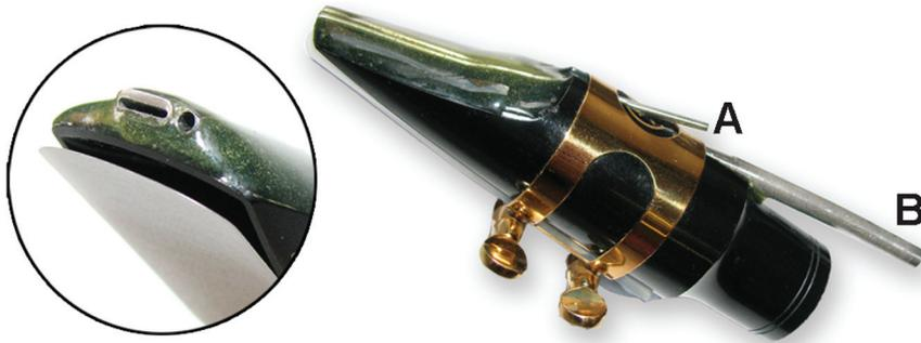
FIG. 3. (Color online) Right: Photograph of the tenor saxophone mouthpiece modified to measure the acoustic impedance in the player's mouth during performance. Tube A is attached to the microphone while tube B is attached to the calibrated acoustic current source. Left: The circular inset shows a close-up of the mouthpiece tip, where the circular end of tube A and the rectangular cross section of tube B are visible just above the reed.
