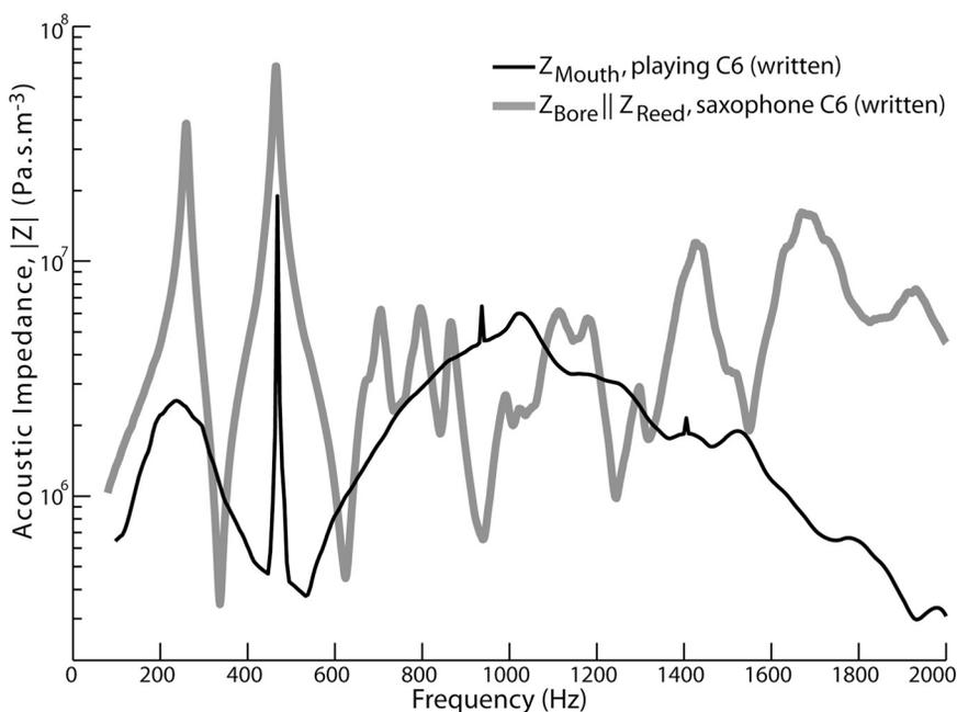
FIG. 4. Impedance measured in a saxophonist's mouth,  $Z_{\text{Mouth}}$  (dark line), while playing the written note C6 (sounding A#4, 466 Hz) and the input impedance of the tenor saxophone,  $Z_{\text{Bore}}$ , shown with the reed in parallel,  $Z_{\text{Bore}} \parallel Z_{\text{Reed}}$  (pale line) for that fingering. Sharp peaks in  $Z_{\text{Mouth}}$  at 468, 937, and 1405 Hz indicate harmonics of the sounded note emitted into the player's mouth.
