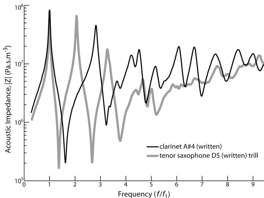
FIG. 1. The magnitude of the acoustic impedance, on log scale, of the clarinet and tenor saxophone ( $Z_{\text{Bore}}$ ), shown for fingerings producing the highest notes of the first register for the clarinet (written A#4, 415 Hz, 16 semitones above the lowest note) and tenor saxophone (written D5, trill fingering, 262 Hz, 14 semitones above the lowest note). To facilitate comparison, the frequencies are scaled to  $f_1$ , the sounding frequency in each case.
