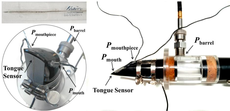
FIG. 1. (Color online) Photograph of the clarinet reed, mouthpiece, and barrel modified to measure tongue contact, mouth pressure, mouthpiece pressure, and barrel pressure during performance. The circular inset at bottom left shows a close-up of the mouthpiece tip, where the tongue sensor (reed with a wire glued on its axis) and the two pressure transducers are visible. A photo at top left shows the modified reed.
