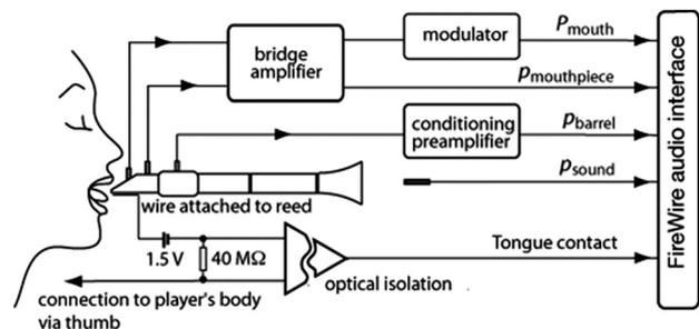
FIG. 2. A schematic diagram (not to scale) shows how tongue contact, mouth pressure, mouthpiece pressure, and barrel pressure are measured during performance.
