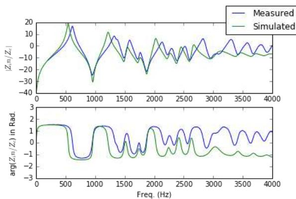
**Figure 7** Measured input impedance of the oboe used in the previous experiment. The impedance corresponding to the modal decomposition used in the simulation in this section is plotted in green. This has a reed compliance added in parallel to correct for the reed, which was absent in the measurement.
