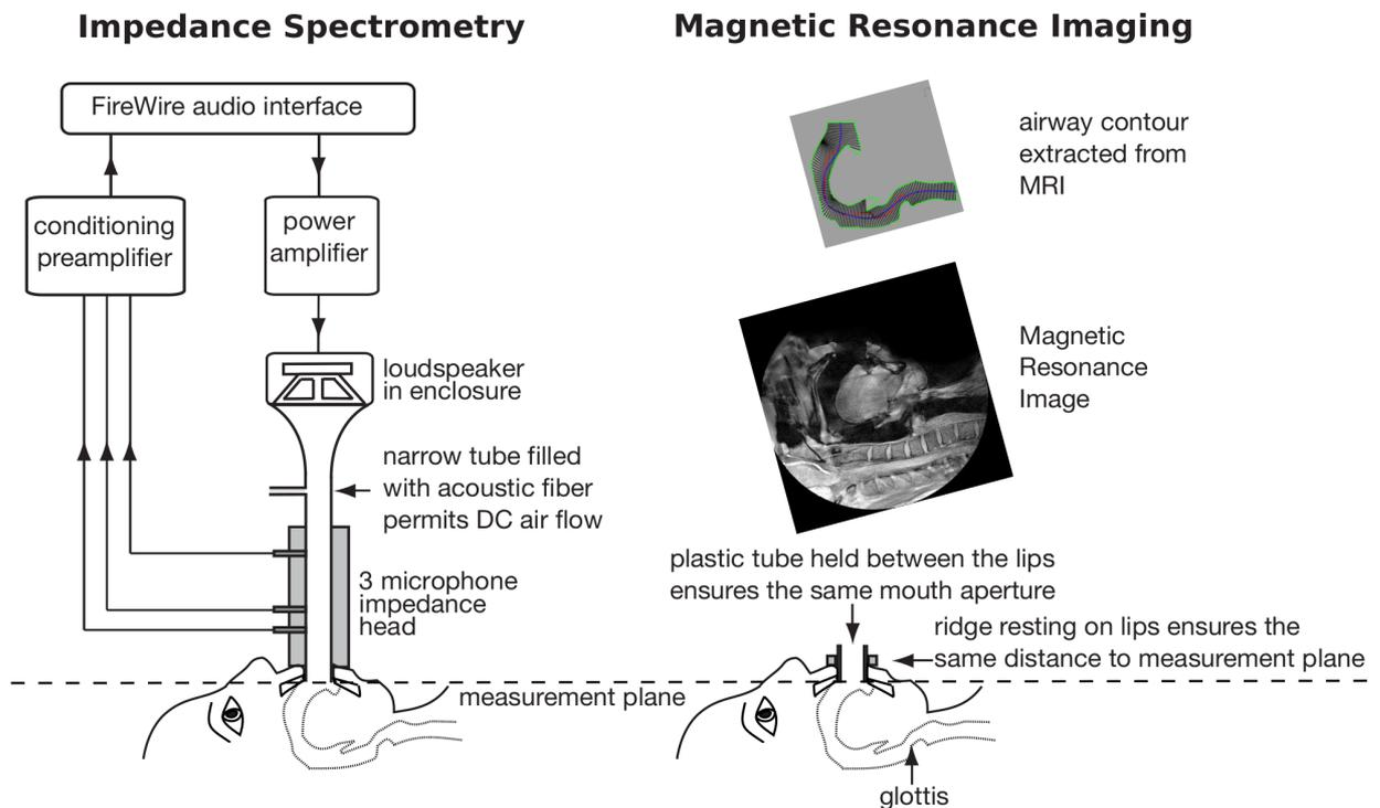
Figure 1: Schematics illustrating the experimental configurations
