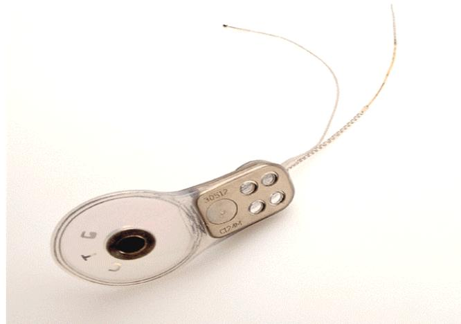
**Figure 1-4 Cochlear implant, showing coil, magnet, case housing the integrated circuit, and electrodes on silicone tube. The case and coil are approximately 55mm in length.**
