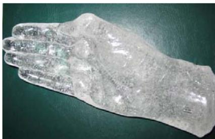
**Figure 1.** Replica of a horn player's right hand in playing position. It was made from synthetic ballistics gelatin.
