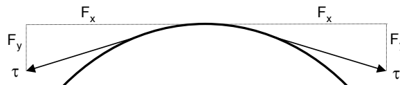
Figure 4.14: Forces in x- and y-direction on a string when a wave travels along the string.
